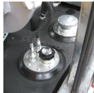
Fuel tank Corrosion-free, 140 litre, high-density polyethylene (HDPE) fuel tank, located in base of frame.
